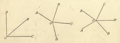
measure all the angles resulting from the combination of the lines two by two. Thus for three lines OA, OB, and OC, the angles AOB, AOC, and BOC should be observed; for four lines six angles should be measured, namely, AOB, AOC, AOD, BOC, BOD, and COD; in general for n lines the measurements should be distributed over  $\frac{1}{2}n(n-1)$  angles. If about 5 series are thought necessary for one inde,
